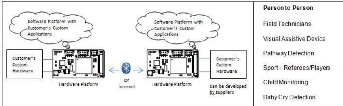
Third configuration is probably the most common IoT application which is a device to an application on a smartphone or a tablet as shown in Figure 4. The smartphone communicates the device through either internet or Bluetooth technology. A common application is when a smartphone receives video relay service (VRS) call, the smartphone notifies the person through the device such as a flasher.
